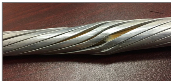
Figure 2 - Strand Loosening Due to Core Damage
