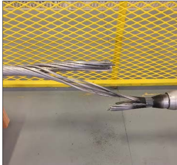
Figure 5-11 Conductor broke just out of epoxy fitting and seating in fitting – Burndy new dead-end
