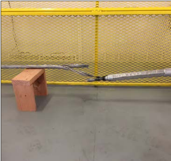
Figure 5-12 Conductor break – Burndy dead-end 1
