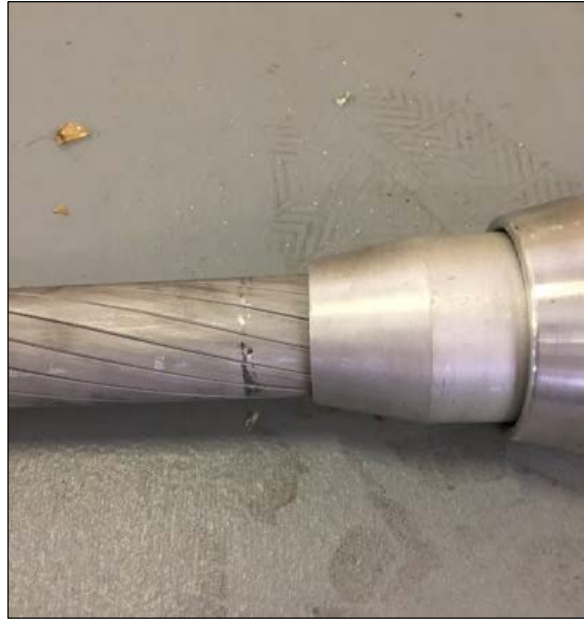
Figure 5-11 Conductor broke just out of epoxy fitting and seating in fitting – Burndy new dead-end
