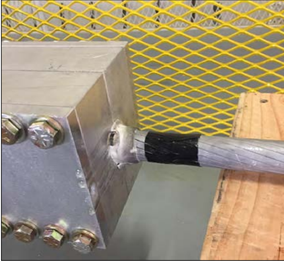
Figure 5-5 Epoxy conductor slippage – AFL new dead-end
