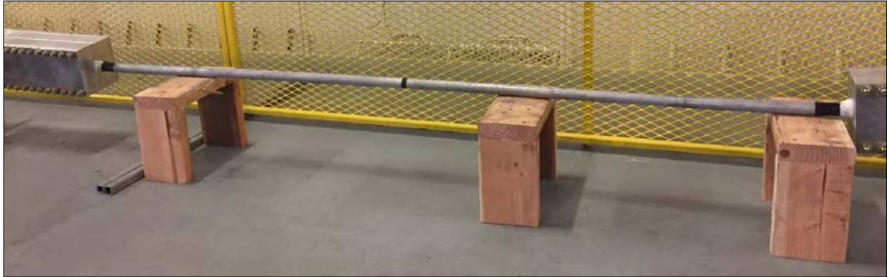
Figure 5-1 Conductor sample in tensile test bed
