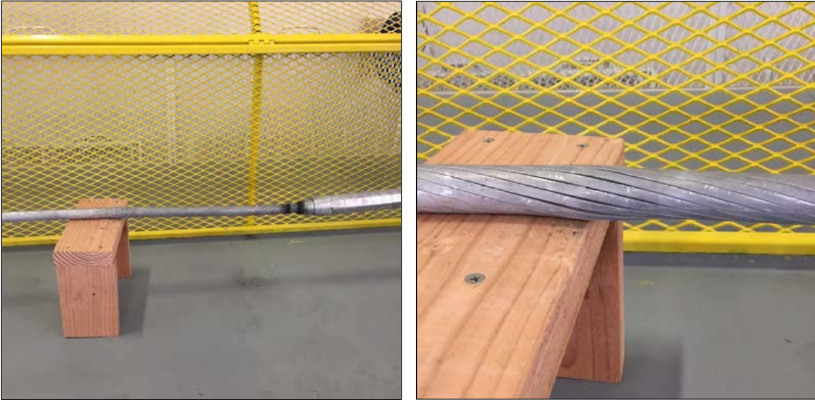
Figure 5-13 Conductor break – Burndy dead-end 2
