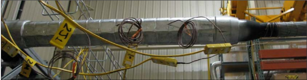
Figure 3-2 Example of the thermocouple placement
