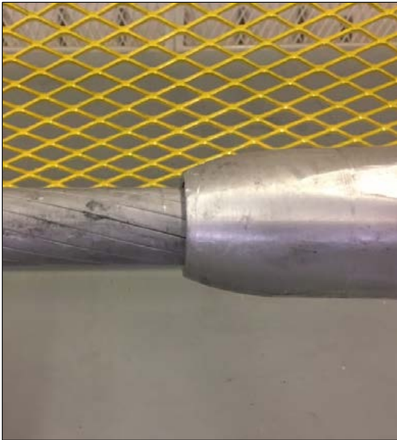
Figure 5-2 Conductor pullout from the Epoxy Fitting – AFL new splice
