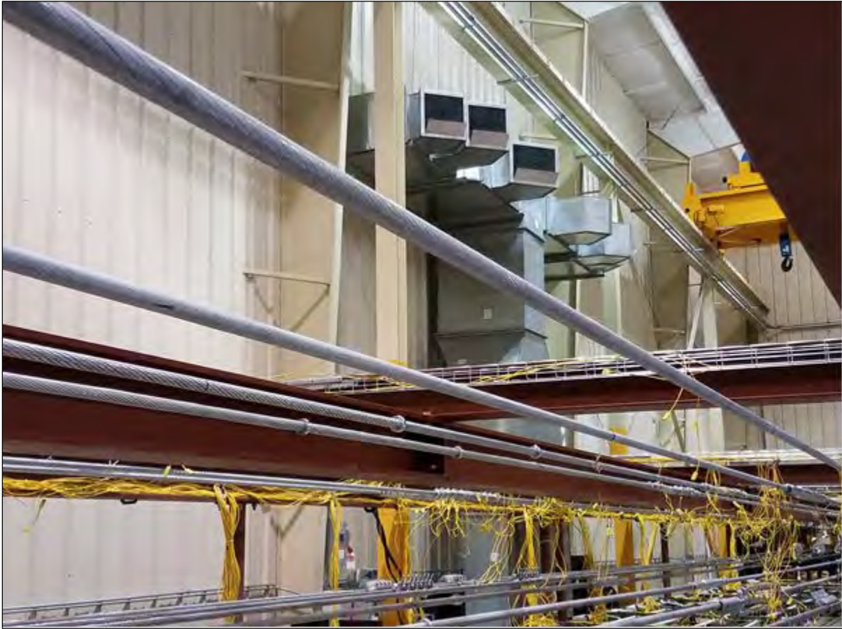
Figure 6-1 Two ACCC conductors after 1500 cycles (the two conductors on the right hand side)
