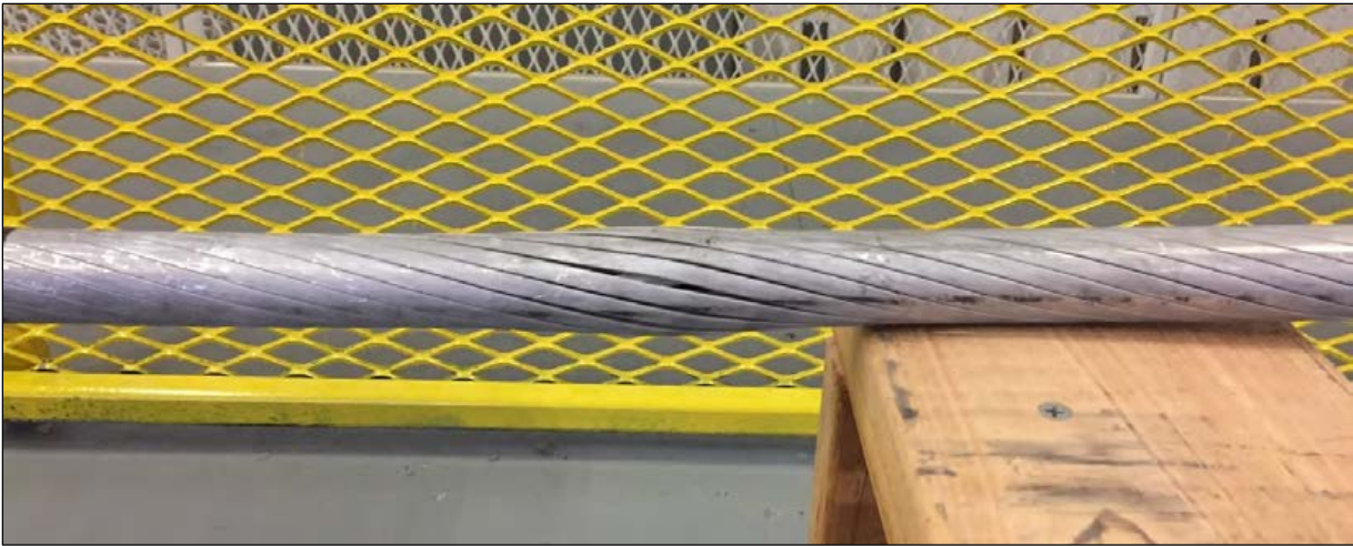
Figure 5-10 Conductor break – Burndy splice 2
