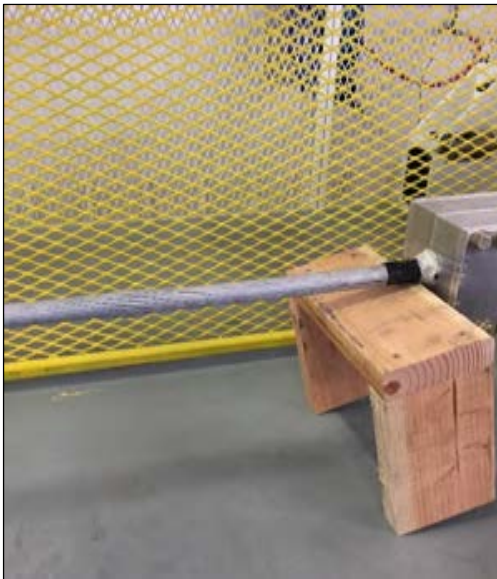
Figure 5-9 Conductor pulled out of splice – Burndy splice 1
