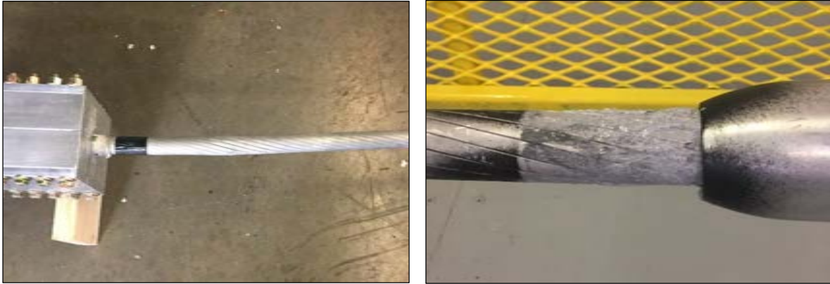
Figure 5-7 Conductor pulled out of dead-end – AFL dead-end 2
