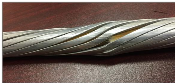
Figure 2 - Strand Loosening Due to Core Damage
