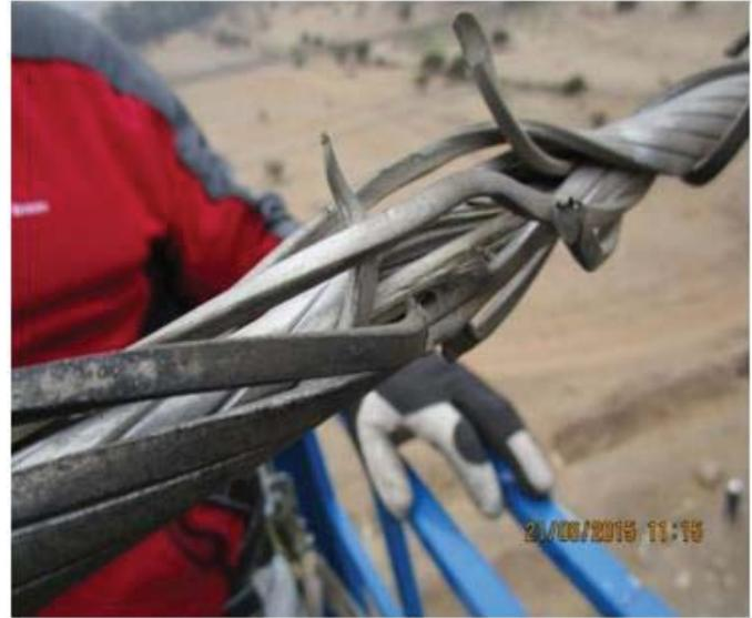
Fig. 3 - lab tests and field observation demonstrate 'load path redundancy' of ACCC Composite Core
