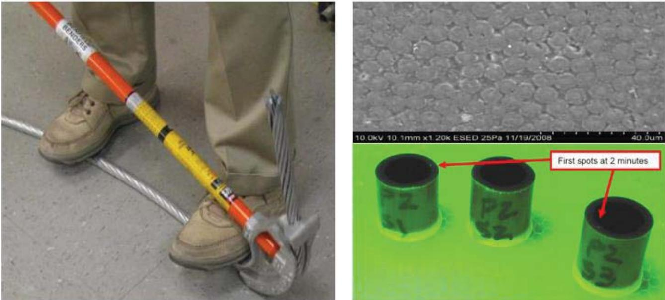
Fig. 2 : ACCC Core bent to 90 degrees with no remarkable damage
